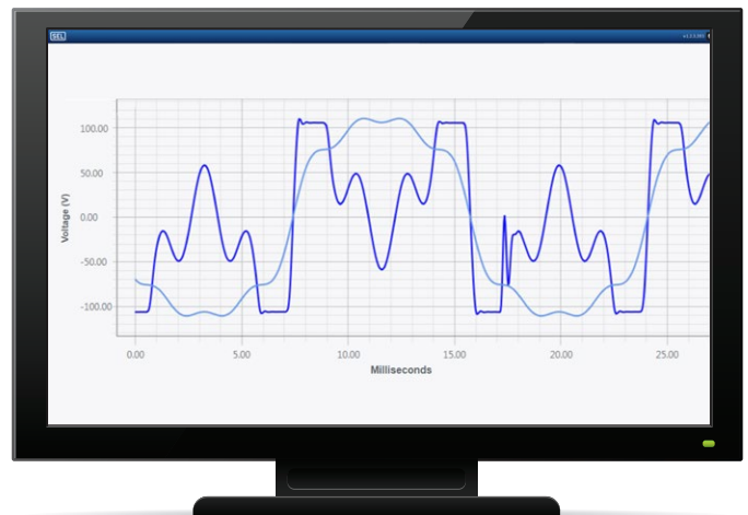
Waveform capture from Wave View, available in the acSELErATOR QuickSet® SEL-5030 Software HMI.
